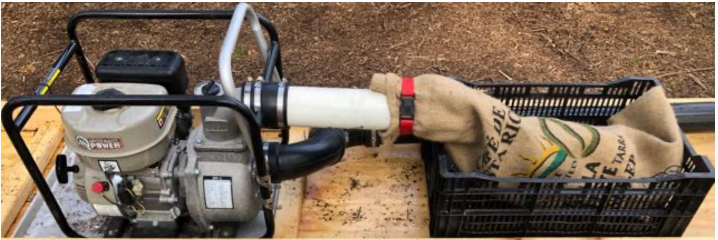
6.5hp, 200+ gpm pump Inlet (black) Outlet (white) Harvest bag/harvest basket/drainage tray
