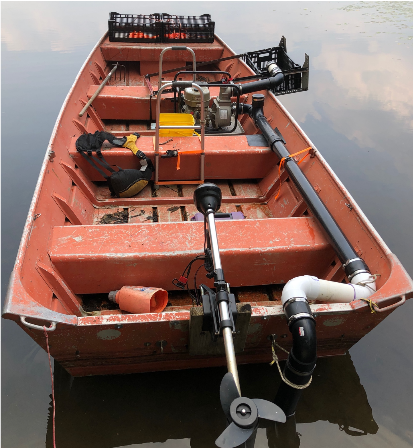
1648 jon boat AVCH powered by a 12v 55 pound thrust trolling motor employed to harvest SAV with a 3" hydraulic pump.
